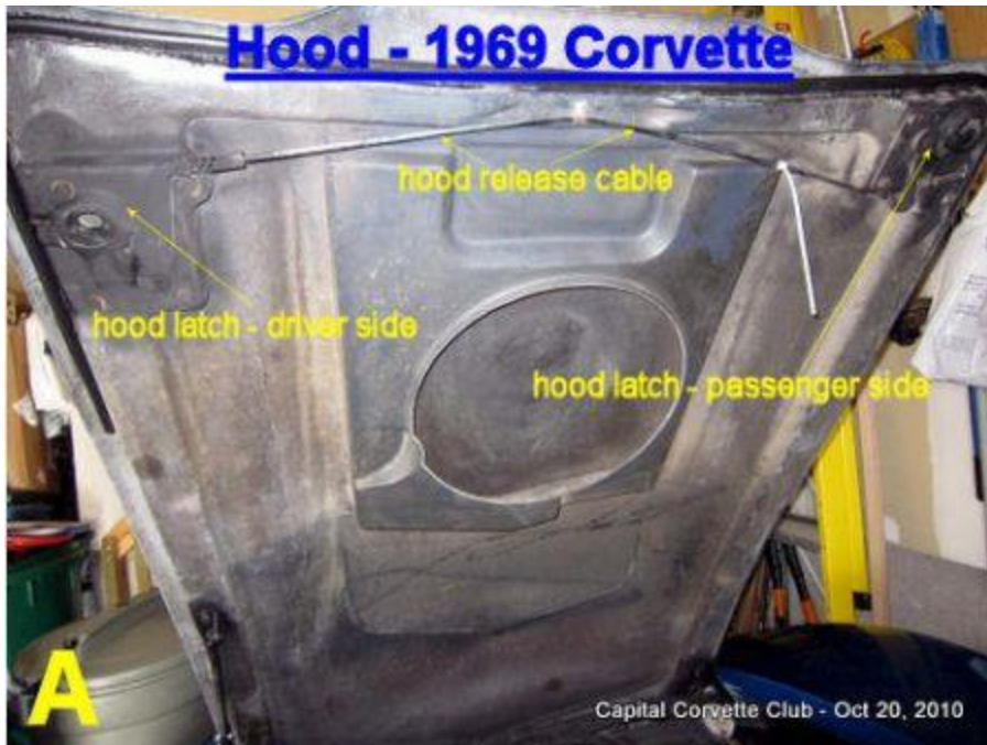
Overview of hood latch components and under hood connecting cable.
