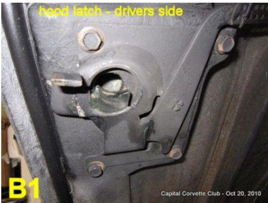
Close up of hood latch on drivers side (locked position).
